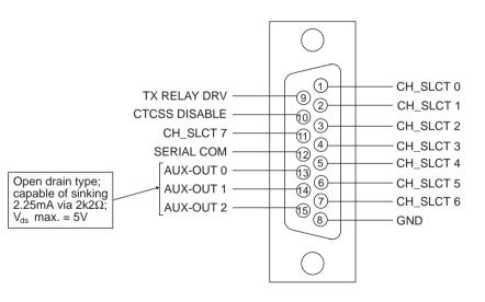
Figure 2.3 T856/857 D-Range 1 Wiring - Rear View
