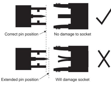
N-Type Plug and Socket Cross-section
